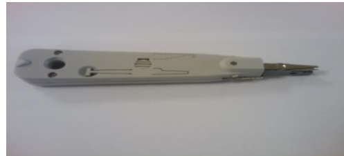
Fig 2. Tool for terminating wires to bifurcated IDC terminals.
