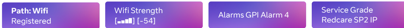
Figure 5 – Typical display cycling on a fully commissioned unit using a wi-fi connection
