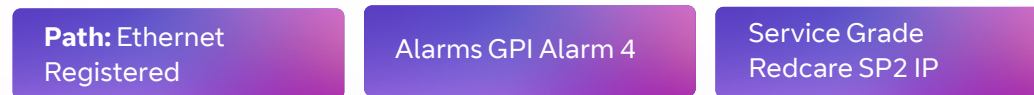
Figure 6 – Typical display cycling on a fully commissioned unit using a wired Ethernet connection
