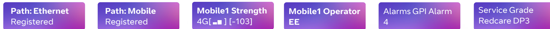
Figure 6 – Typical display cycling on a fully commissioned unit with a good signal strength and Pin 4 in the alarm or open state
